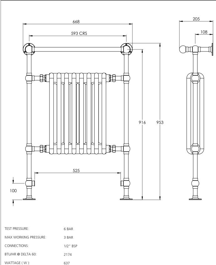
THIS LEFROY BROOKS RAIL IS SUITABLE FOR CLOSED CIRCUITS ONLY DIMENSIONS IN MILLIMETRES
