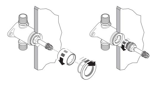
$XO4220 - \frac{1}{2}$ " x  $\frac{1}{2}$  turn (clockwise closing) ceramic cartridge including plastic adapter – PXT027  $XO4224 - \frac{3}{4}$ " x  $\frac{1}{2}$  turn (clockwise closing) ceramic cartridge including plastic adapter – PXT033
