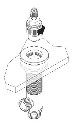
Pair of replacement 1/2 turn ceramic cartridges - PXT014
