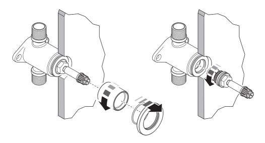
XO4219 – <sup>3</sup>/<sub>4</sub>" x <sup>1</sup>/<sub>4</sub> turn (clockwise closing) ceramic cartridge including plastic adapter – PWV099
