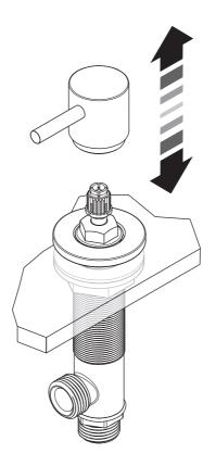
Pair of replacement plastic spline adapters – PXT006
