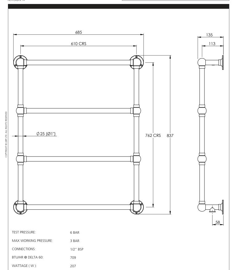
THIS LEFROY BROOKS RAIL IS SUITABLE FOR BOTH OPEN AND CLOSED CIRCUITS
